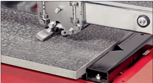
Special design for cutting 20 mm ceramics.
