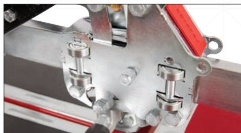
Cutting handle consists of 13 roller bearings.
